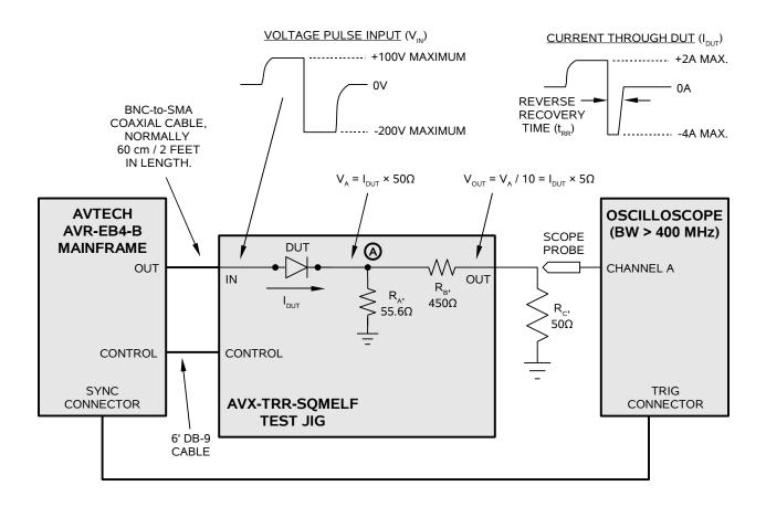
A 50 Ohm resistance (R<sub>c</sub> in the diagram above) must be connected to ground on the output. This can be a discrete resistor, a feed-through terminator, or the input impedance of an oscilloscope. If a high-speed sampling oscilloscope is used, the input should be protected by adding attenuator on the input.
